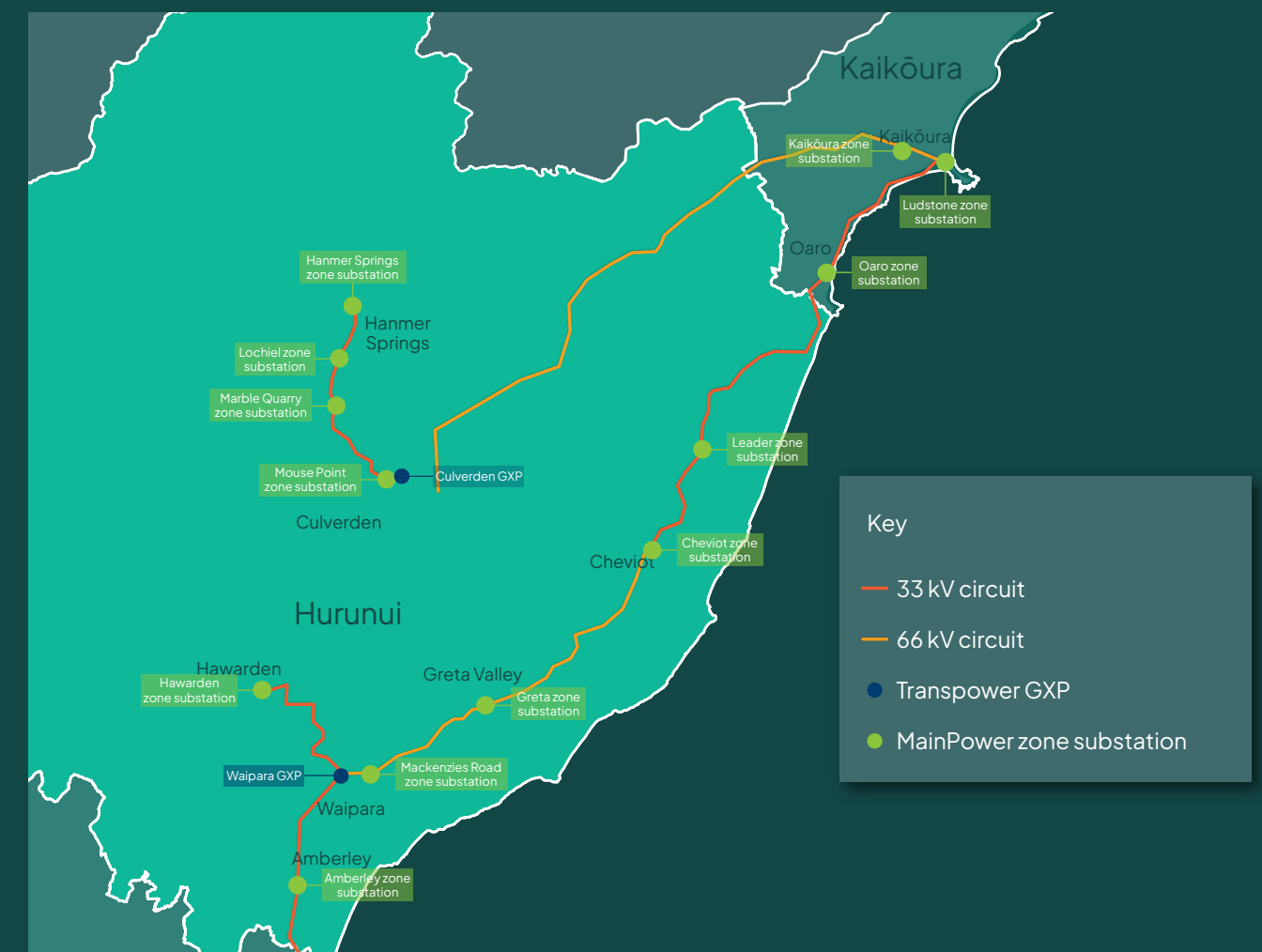
Figure 4.6 Hurunui subtransmission network
