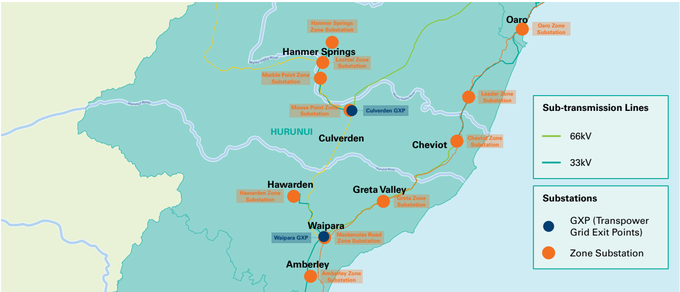
Figure 6.7 Hurunui sub-transmission network (existing)
