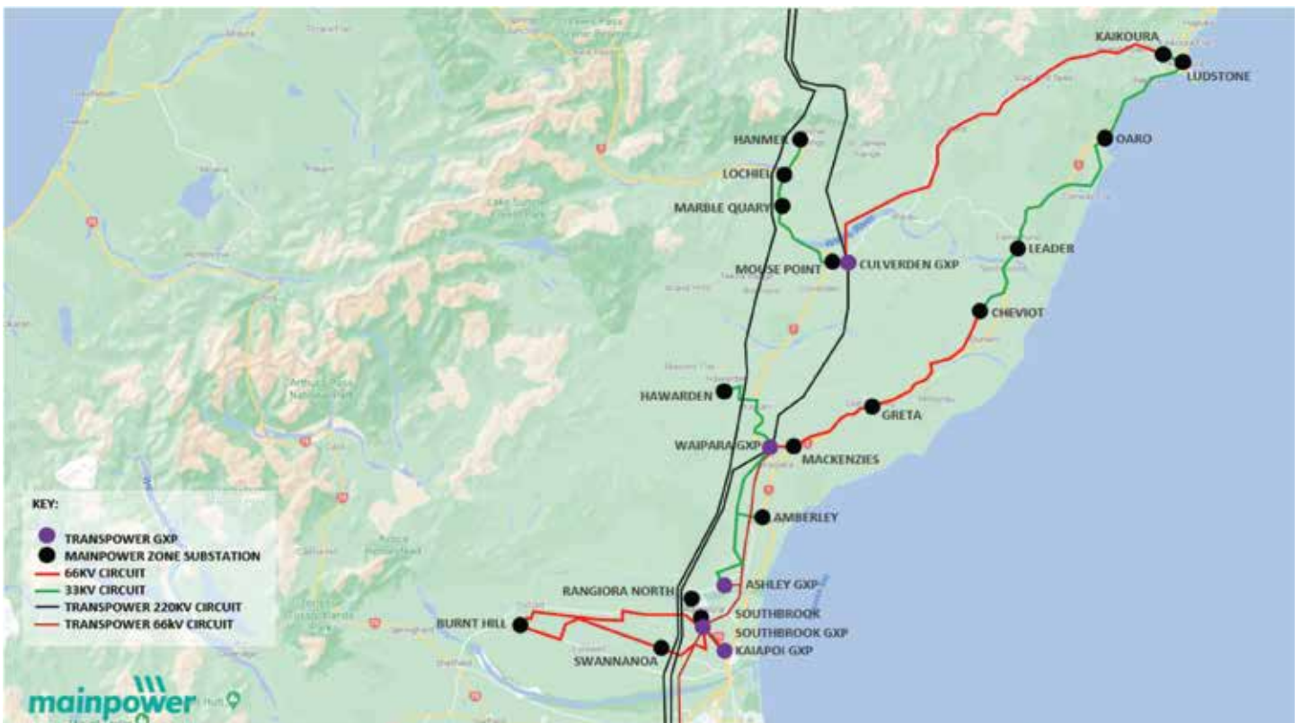
Figure 5.3: MainPower’s sub-transmission network
