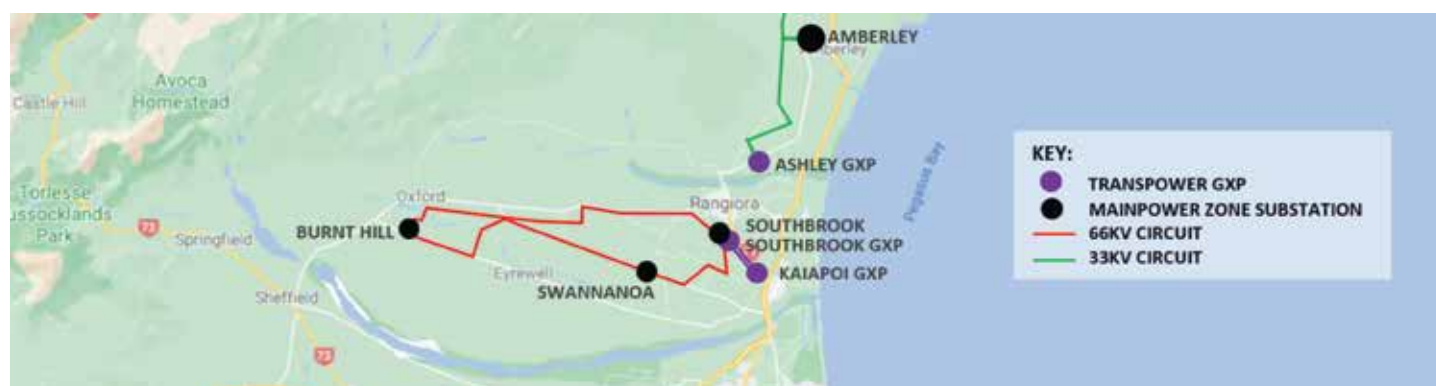
Figure 6.6: Waimakariri region sub-transmission network (existing)
